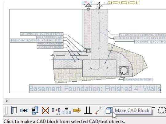
7. Now, group select both upper and lower CAD blocks and use **Make CAD Block**
