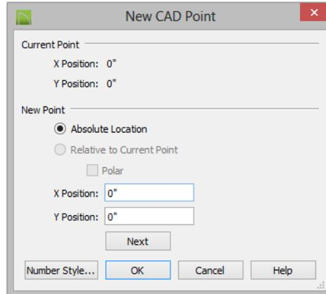
2. Select **Absolute Location** and define the point's position at (0,0) and click **OK**. This is the current point that serves as the Start Point for the first line of the plot plan. See “Point Tools” on page 1054 of the Reference Manual.
