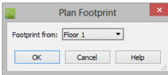
2. Select a floor, then click **OK** to create a CAD object representing the building footprint in the CAD Detail window. See “Plan Footprint” on page 1099 of the Reference Manual.
