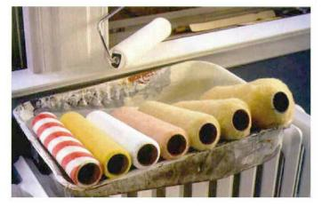
There are several factors I consider when choosing a roller pad (photo above). The first is the surface I'm going to paint. For smooth surfaces, a roller pad with a short nap (¼ in. to ½ in.) is fine. But if you're covering a heavy stucco, you may
