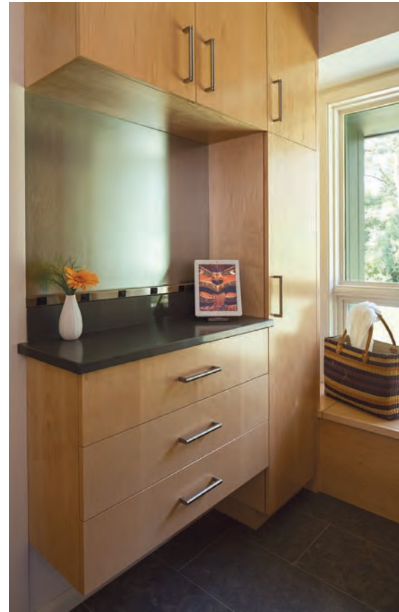
Sophisticated mudroom. Carved from the inside of the garage, the new 6-ft. by 12-ft. mudroom offers plenty of storage and a bench for putting on shoes. The large window and maple cabinets give the small space a lightness that contrasts with the dark-gray tile floor and countertop. The counter includes a half-dozen outlets for charging electronics.
