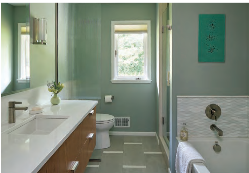
Revamped bath. Keeping fixtures in their original locations and converting what was a hall closet at the end of the tub into a shower kept costs down for the bath remodel. The ribbed-glass partition next to the vanity was inspired by a partition wall with a ribbed-glass window that was in the same spot in the original bathroom.
